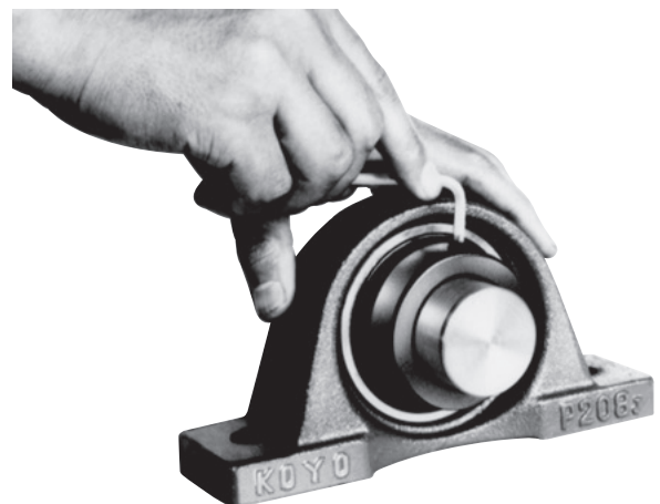
Fig. 14.10 Installing eccentric locking collar
